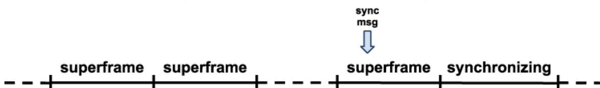
Figure 24: Synchronization on the receiving node.
