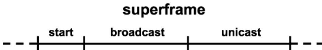
Figure 20: Structure of the superframe.
