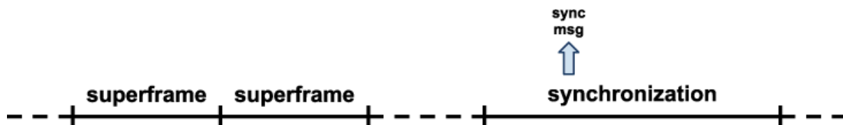
Figure 23: Synchronization on the sending node.
