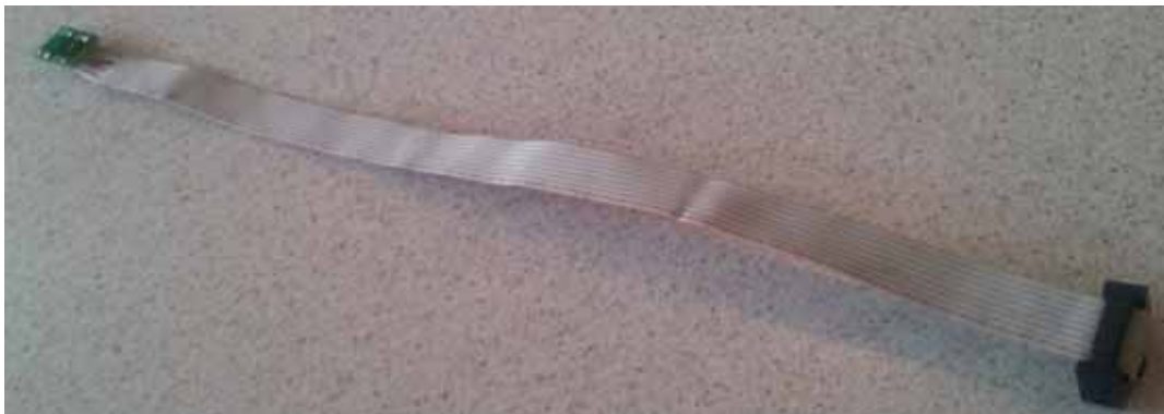
Figure 30: Thermal-Sensor for the BeagleBoard Trusted Sensor (proof of concept)
