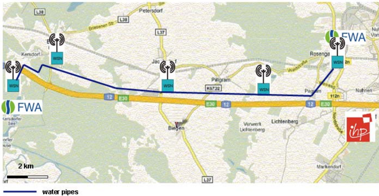
Figure 15: Map of the FWA demonstrator with position of the measuring nodes. Data should be delivered to the top right FWA head station.
